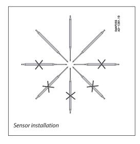
The charge is a mix of liquid and gas. Due to the mixture of liquid and gas the sensor must be installed in an area or environment that is warmer than the valve.
