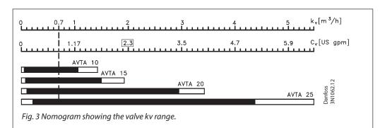
$K_{\rm v}$  values are always given for water flow in  $[m_{\rm 3}/h]$  with a pressure drop  $\Delta p$  of 1 bar. The valve should be selected so that the necessary  $k_{\rm v}$  value lies in the middle of the regulation range.
