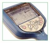
Built for on-site use – IP65 Shock resistant, ingress protected
