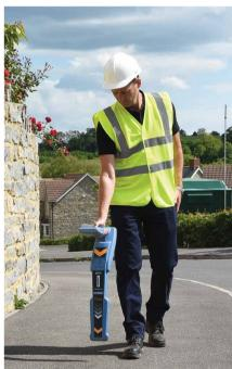
RD8100, our most advanced precision locator range, is built on this pedigree for performance, quality and durability. Containing a unique arrangement of 5 antennas, it allows you to choose the optimum level of precision for the job in hand. Integrated GPS and usage-logging options automatically generate data for customer reports, or in-house quality and safety audits to promote best working practices.
