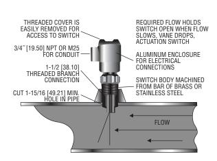
Threaded Branch Connection Installation. May also be installed using tee, flange or coupling.
