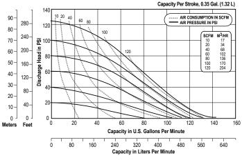
NOTE: Performance based on the following: PTFE fitted pump, flooded suction, water at ambient conditions. The use of other materials and varying hydraulic conditions may result in deviations in excess of 5%.
