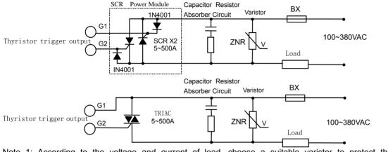
Note 1: According to the voltage and current of load, choose a suitable varistor to protect the thyristor. A resistor-capacitor circuit (RC circuit) is needed for inductance load or phase-shift trigger output. Note 2: SCR power module is recommended. A power module includes two SCRs, is similar to the above dashed square.
