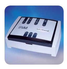
The IRiM (infrared interface modul) uses modern infrared technology to transmit measurement data from the MD 600 photometer to one of 3 optional interfaces. These interfaces can be used to connect to a PC, a USB printer<sup>1)</sup> or alternatively a serial printer<sup>2)</sup>. The interface which is selected is displayed by an LED function indicator. The user can switch between the interfaces using the "Select" button.
