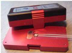
Calibration of Pressure Indicator Low Pressure version at 25 N/cm 2
