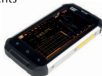
The Table View showing Instantaneous, Valley, Average and Peak, plus the unique Meltmaster temperature (on the 055 L model) readings.
