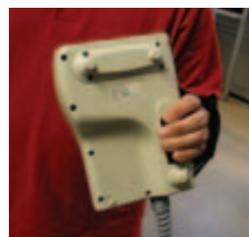
Panel assembly of JSHD4H2 on a programming unit for robots.
