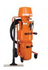
Air powered ejector vacuum cleaners have no moving parts, motors or pumps. They do not require electricity and provide enormous advantages for demanding operations in industry, shipping and offshore. They are used to collect any industrial product or material (liquids, dusts or granules) that can be conveyed along a suction hose.
