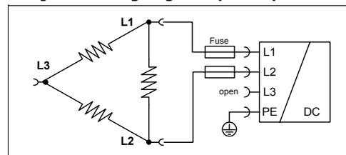
Fig. 27-8 **2-phase operation, allowed output current**
