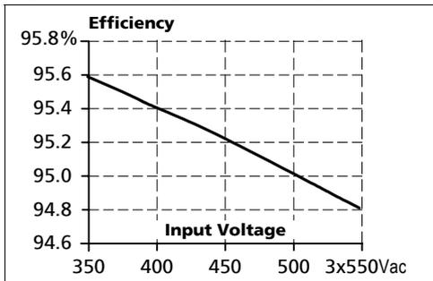
Fig. 11-4 Losses vs. input voltage, 48V, 10A
